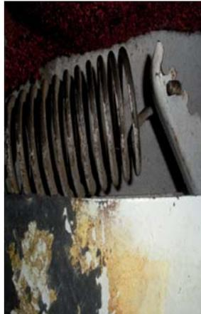
(this is why it's a good idea to remove one of the seats) and close the top until it latches. At this point the springs are extended as far as possible. Using the square  $\frac{1}{4}$ " pieces you cut earlier slide each of them as far as you can into the space between each coil of both springs. Release the latch while holding on to the top and slowly let it open while watching the square pieces to make sure they don't fall out of the spaces between the coils.
